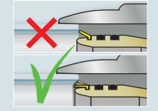
The Protector Ring prevents insertion of non-calibrated pipes.
