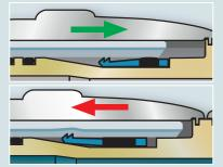
When the calibrated pipe is inserted the Grip Ring gives way. The Grip-Ring is embedded into the connection.
